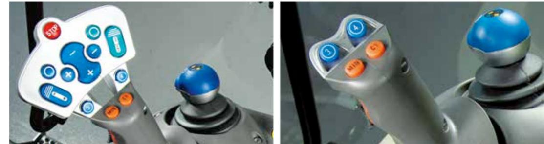
The armrest folds up to expose a rotary control that selects the button assignment for the multi-function joystick. The oil flow volume of the individual valves can be set with the rotary controls.
