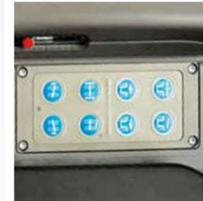
➡ The crossgate lever controls the 1st and 2nd valves sensitively. The 3rd and 4th hydraulic circuits are controlled with the buttons on the crossgate lever.
