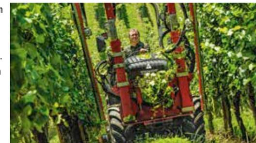
When cutting leaves, the suspension with anti-roll control dampens uneven ground reliably and sensibly with FSC. It ensures that working height and lateral tilt remain constant. Advantage for the driver: calm, relaxed work, because constant adjustments are not needed.
