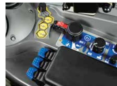
The 3rd and 5th control units can be actuated with the three linear modules on the armrest.
