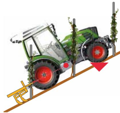
The smallest turning radius is just 3.2 metres, depending on the tyres. You will notice this immediately at the end of the row, where you can switch to the row after the next without having to change direction.
