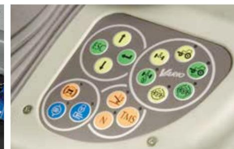
On the dashboard, you can quickly and easily operate the multiple display, comfort engagement for 4WD, differential lock and front axle suspension as well as the Tractor Management System TMS.
