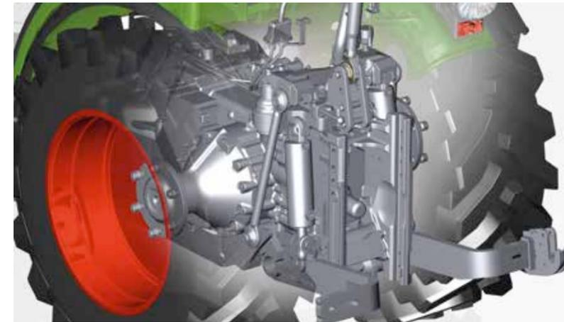
➡ You can control the lateral and tilt adjustment of the swinging power lift, as well as swing and lock, with the push of a button. You can monitor tilt with the tilt control indicator in the cab.
