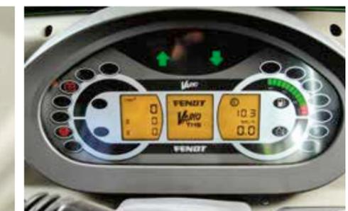
The clearly laid out instrument cluster has a speed display with cruise control, rpm display and multi-display.
