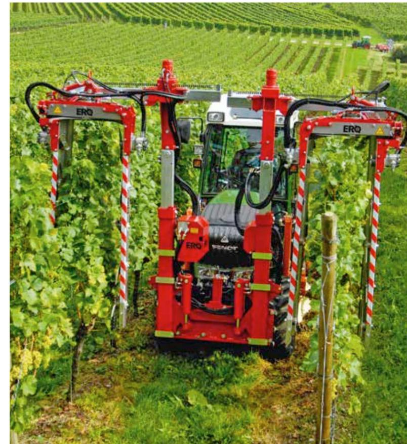
↻ The lower links can be adjusted to the right and left using two hydraulic cylinders. Swinging to both sides is possible in floating position. The rear implement is guided precisely in the row.
